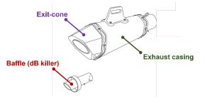
**Tamper-proof** = an exhaust is considered tamper-proof when grinding, cutting or drilling is required to remove an exit cone, a fastener or a baffle from a silencer.
