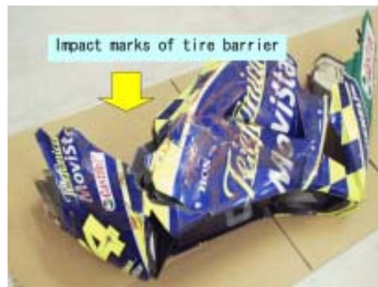
(Figure 5) Damage of the vehicle (front fender)
