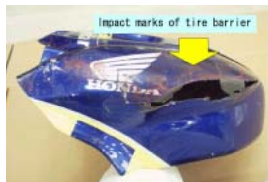
(Figure 7) Damage of the vehicle (tank shell)
