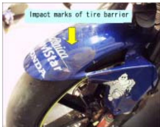
(Figure 6) Damage of the vehicle (front cowl)
